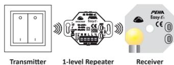
In 1-level operation, a radio signal received from a radio transmitter will be passed on to the respective receiver. The receiver cannot be cascaded in this mode. Repeated RF signals are not retrieved.
