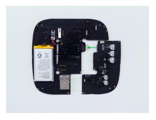
Please note: the board contacts should be plugged in the bottom row of the connector (closest to the board). When connected correctly, the boards are on the same level.
